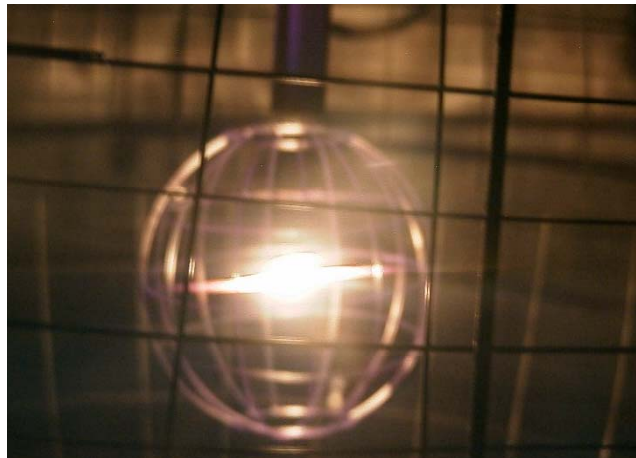
Figure 9.4 Diagwire configuration. The wire is placed along the diameter across the central grid parallel to the ground surface.
