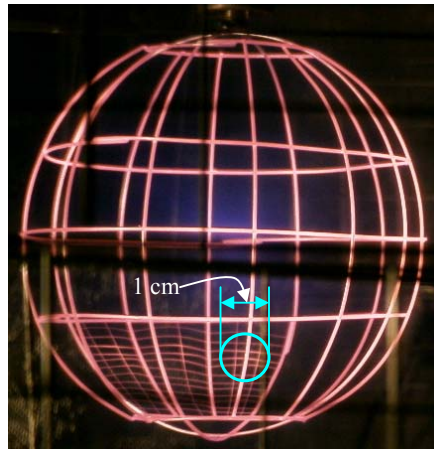
Figure 13.8 Fine wires are introduced on the surface of the grid to intercept the ions leaving the cathode. The dimension of the jet is \sim 1 cm in diameter.
