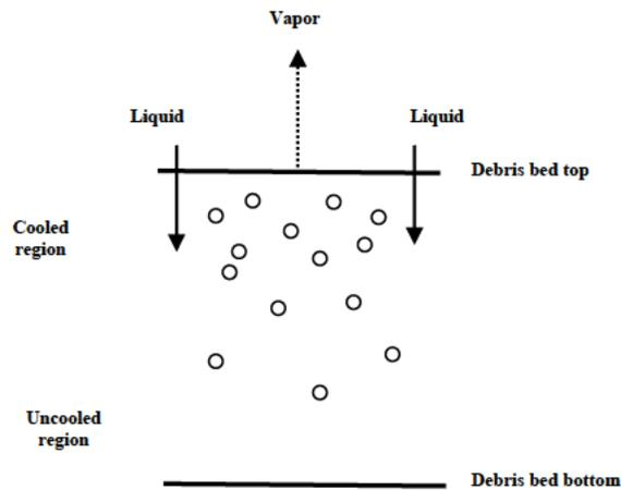
Figure 45. Closed bed debris bed cooling.
