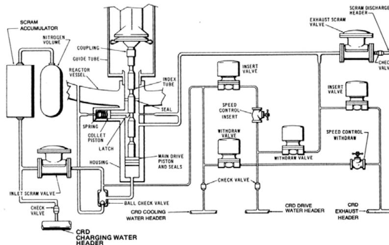
Figure 37. BWR control rod drive mechanism at the bottom of a BWR reactor vessel showing the control rod graphite seals location [2].
