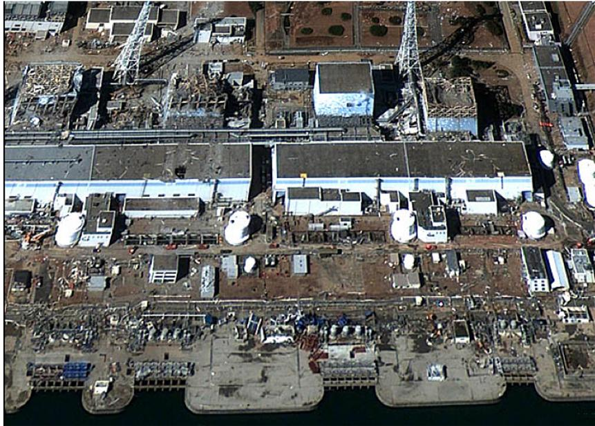
Figure 48. Aftermath of Fukushima Daiichi accident on March 11, 2011, one week after the accident. Rubble from hydrogen explosions in units 1, 3 and 4 and fire in unit 3 is spread over the site. Damage from earthquake and tsunami to the electrical systems apparent along the water front. Steam still emanating from unit 2. Source: DigitalGlobe.
