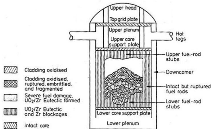
Figure 43. Debris bed resulting from the core damage in the Three Miles Island accident.
