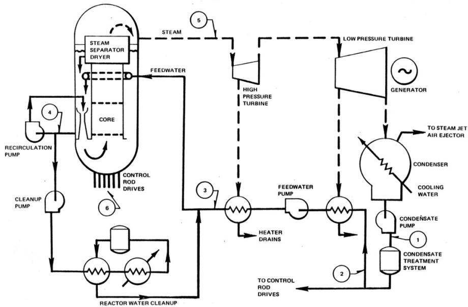
Figure 3. Typical BWR flow diagram. The role of the core spray system in the progression of the accident is undetermined. Source: GE.
