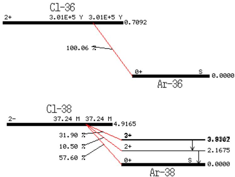
Figure 42. Decay diagrams of the  $\text{Cl}^{36}$  and  $\text{Cl}^{38}$  isotopes.
