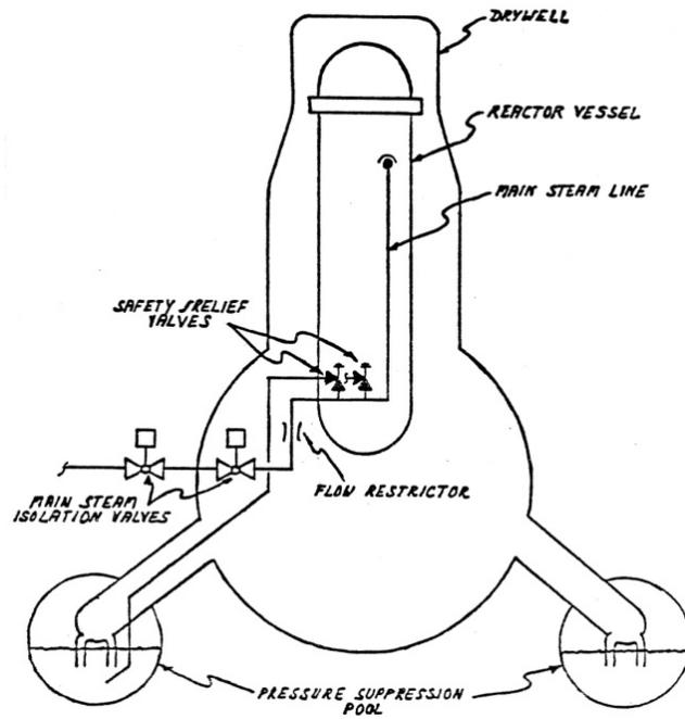
Figure 6. Main isolation valves and safety relief valves used in depressurization of the BWR.
