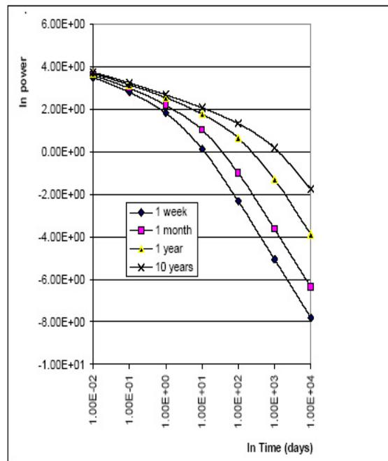
Figure 19. Decay heat power release for a 3,000 MWth Light Water Reactor, LWR for different operational times. The decay heat generation power decreases rapidly within a few days after shutdown.
