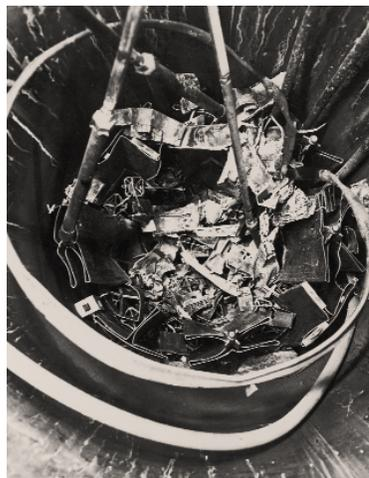
Figure 36. Damaged core resulting from steam explosion caused by a criticality accident in the military Small Low power reactor experiment SL-1 BWR. A worker inadvertently yanked out a
