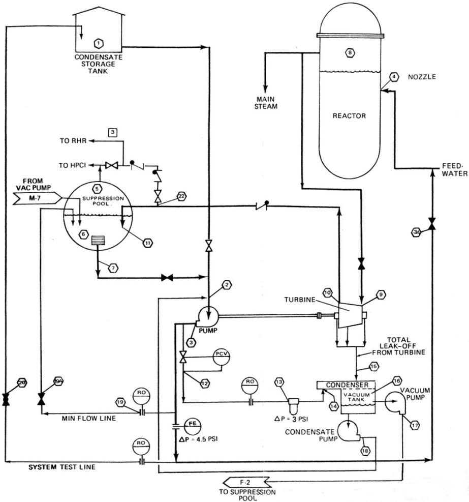
Figure 7. BWR Reactor Core Isolation Cooling system, RCIC. A steam turbine uses steam to drive a pump injecting water drawn from the condensate storage tank into the core. Exhaust from the steam turbine is directed to the pressure suppression pool. HPCI: High Pressure Coolant Injection system, RHR: Residual Heat Removal system.
