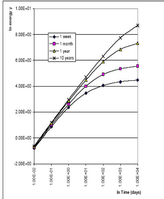
Figure 20. Decay energy or integrated power release after shutdown for a 3,000 MWth LWR for different reactor operational times. If not extracted and rejected, the energy released would result in fuel damage including fission products release and hydrogen generation.
