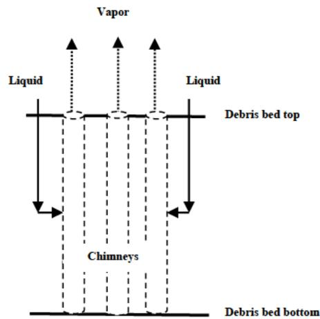
Figure 44. Debris bed chimneys cooling.
