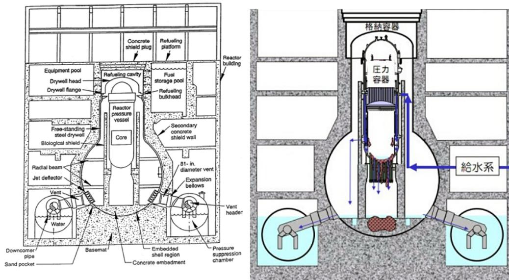
Figure 22. Cutout through containment and turbine hall showing the location of the fuel storage pool in a typical BWR. Plant systems below grade level and hence affected by flooding from the tsunami event include pumps and electrical components. The dry well includes a sump. Any leaking corium material through the control rod seals could interact with the sump water as well as the concrete mat causing a steam explosion, then becoming embedded in the concrete. Source: GE.
