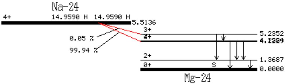
Figure 41. Decay diagram of  $\text{Na}^{24}$ .
