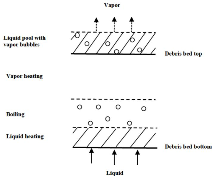
Figure 46. Multilayered once-through debris bed cooling.
