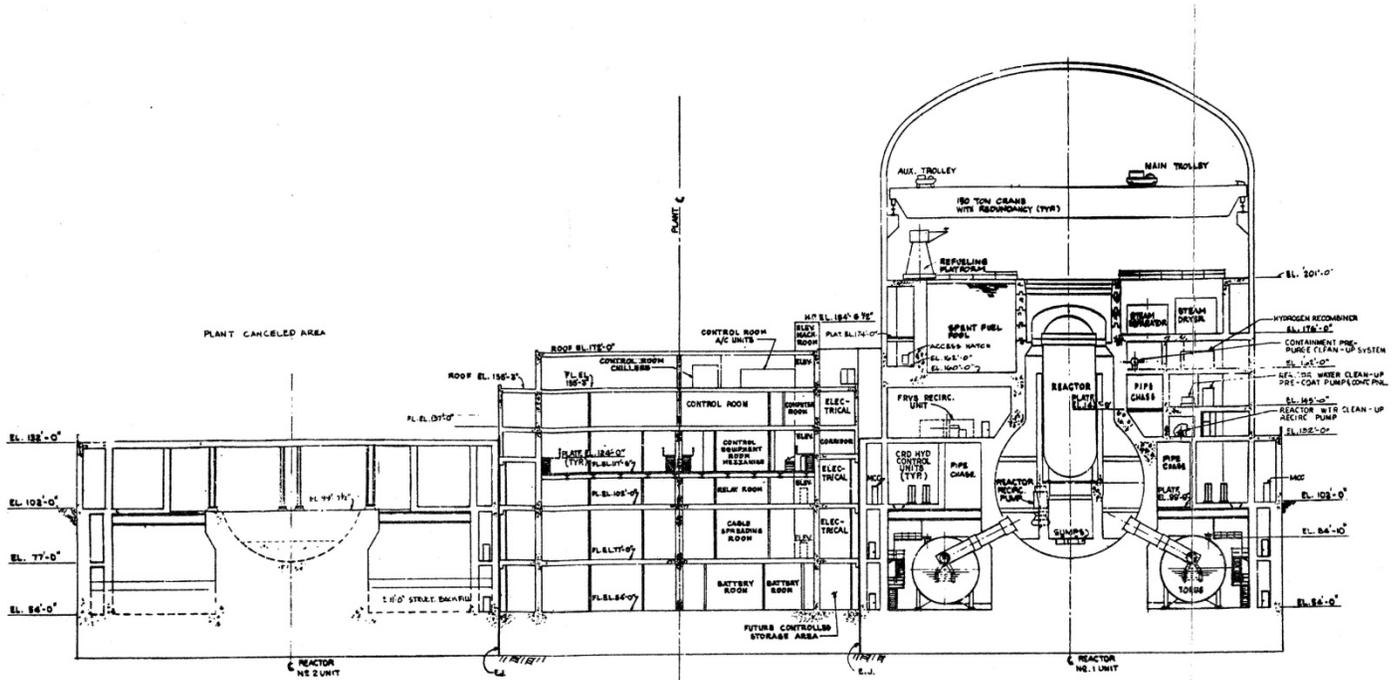
Figure 23. Perpendicular cutout through the containment structure showing the location of the storage batteries. The gate and other connections between the fuel storage pool and the top of the core may have sustained damage as a result of the earthquake and caused leakage of the pools' cooling water. Source: GE.
