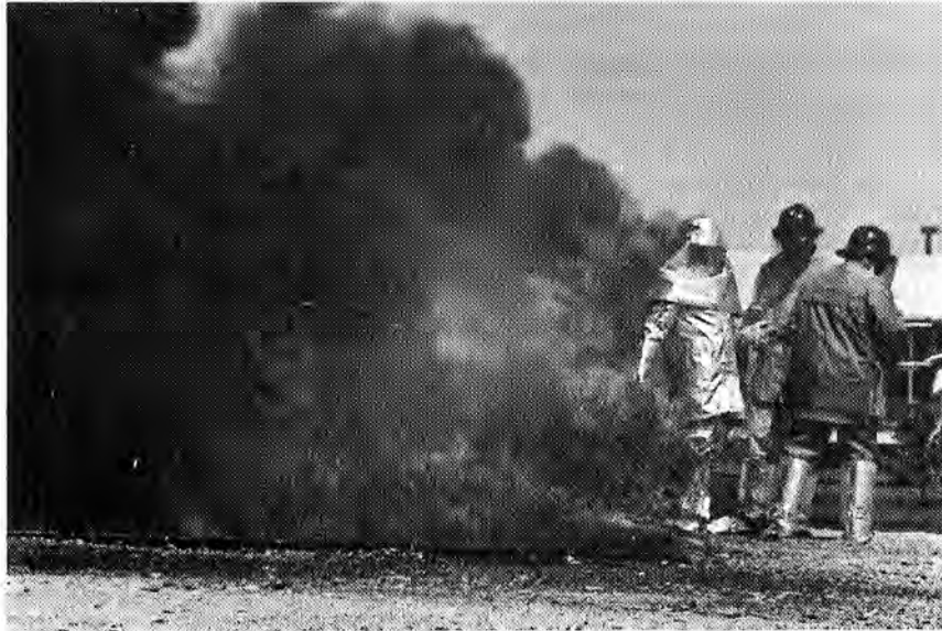
May 6-7; Conference on Materials for Improved Fire Safety, held at MSC, demonstrated NASA-developed technology available to industry. Among materials developed to reduce spacecraft fire hazards, Fluorel could be sprayed on materials to fireproof them against temperatures to 1500 K (2200°F). Fluorel-coated Durette fabric could provide lightweight, durable suits (suits to the right) that would permit firemen to work close to fires. Added aluminum layer would reflect heat outward and provide a vapor barrier to protect firemen from steam. Fluorel sprayed on chair (lower left) charred in the direct flame of a torch but when the material was scraped off the wood was revealed to be undamaged.
