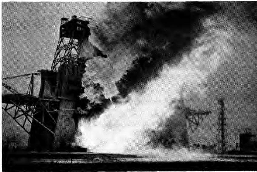
September 30: The 15th and last Saturn V 1st stage (S-IC-15) was successfully captive-fired for 2 minutes 55 seconds at NASA's Mississippi Test Facility. At right, the 14th S-IC stage was photographed on the test stand earlier. The captive tests began May 16, 1967, to flight-certify stages for lunar missions.
