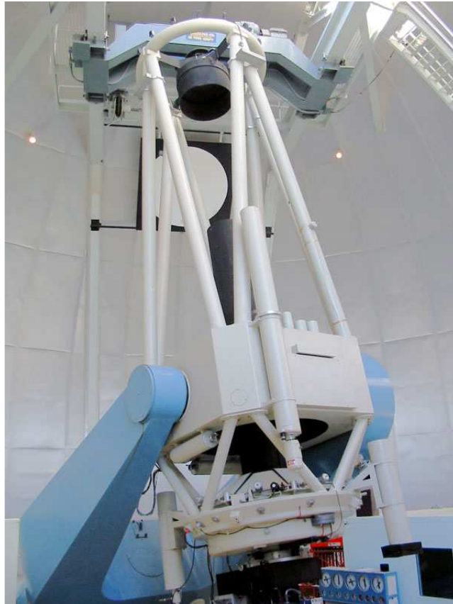
The NOFS 61-inch (1.55-meter) Kaj Strand astrometric telescope (USNO image by Geoff Chester)
