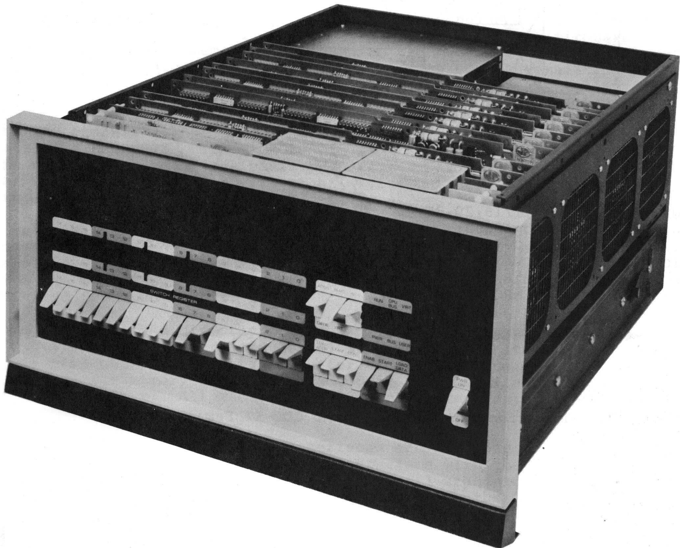
Figure 1. CDP-XI/35 Computer with 80K Words of 8K by 16-Bit, 675-ns Core Memory Modules (Using CDP-16K, 850-ns Core Memory Modules, a Full 128K Works can be installed)
