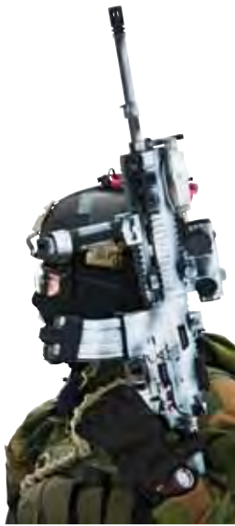
The HK416N went into service with Norway's armed forces in 2010 and replaced the Kongsberg AG-3 (aka HK G3A5) that had been in service since 1967. With its 16½-inch barrel, the HK416N closely resembles the MR556A1 and is typically issued with an Aimpoint CompM4.
