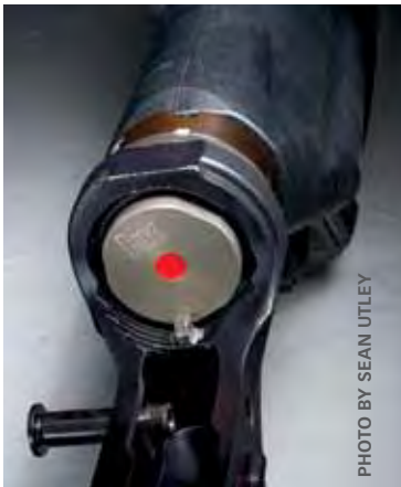
The MR556A1 includes the tungsten-filled buffer that is partly responsible for the high reliability of the HK416. It is designed to slow the bolt carrier during operation and reduce the recoil impulse.
