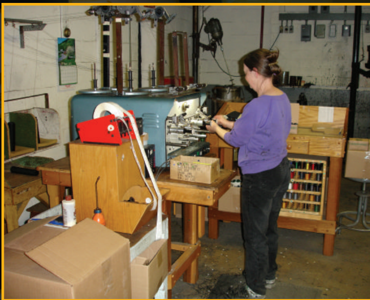
Brownell & Company winds thousands of spools of high quality bowstring and serving material each month. Mary Vachon tends a jig spooler.
