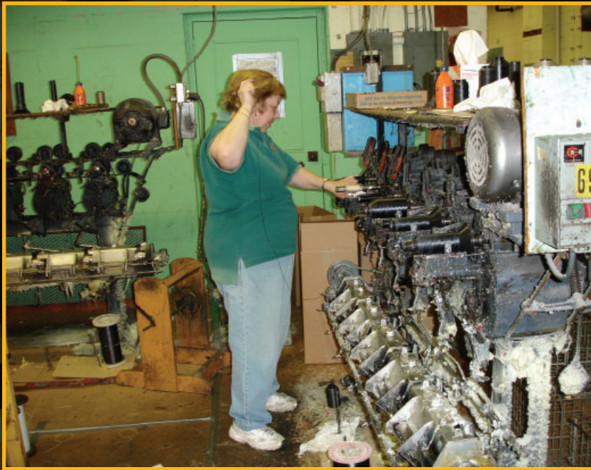
The proper wax prolongs the life of any bowstring. Irene Willard maintains a machine that applies Brownell's proprietary wax to bowstring material.
