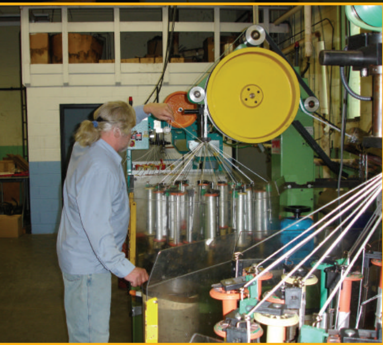
Among Brownell's strongest serving materials are Brownell Crown and Diamondback Serving. Both are braided products. Dean Brown oversees a unique Brownell braiding machine.
