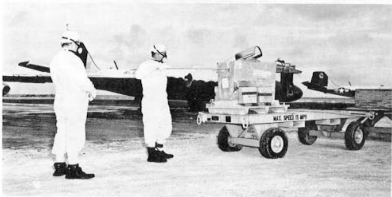
Figure 34. Radioactive filter in lead cave is rolled using long pole before being placed in lead pig, Johnston Island, DOMINIC.
