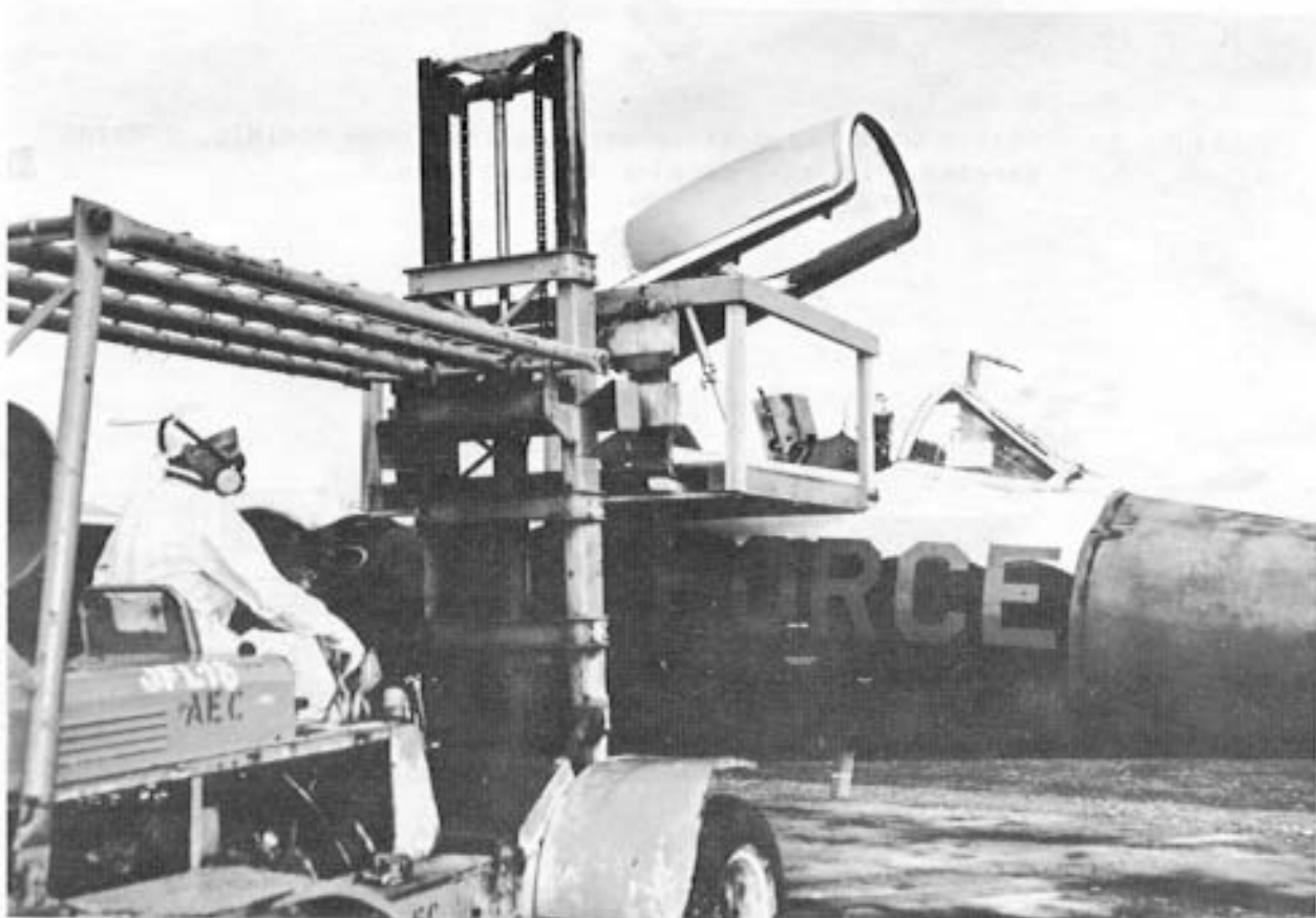
Figure 32. Pilot prepares to leave sampler B-57 via a platform on forklift, Johnston Island, DOMINIC.
