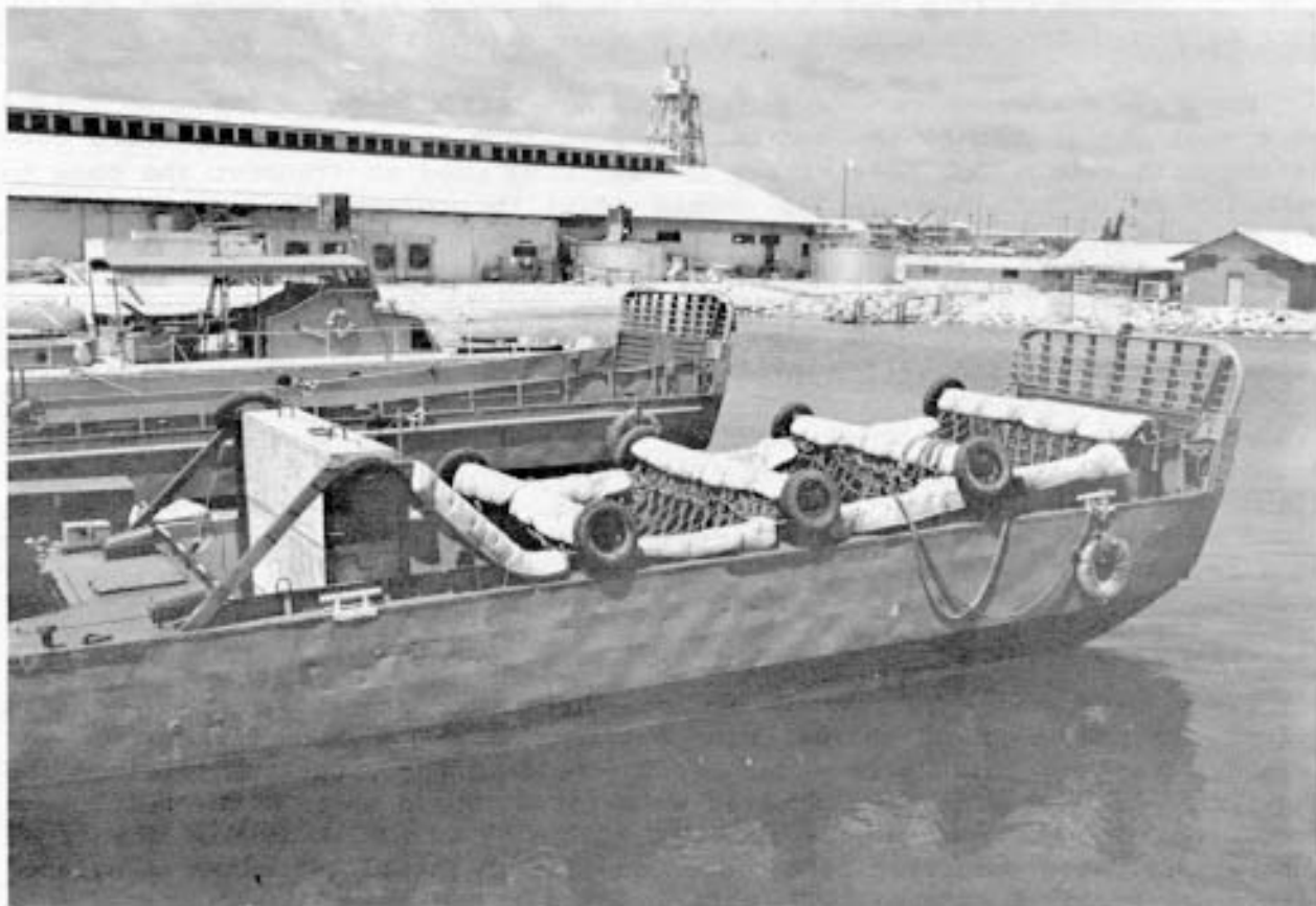
Figure 24. Modified M-boat (LCM) for handling radioactive pods returned to Johnston Island, Operation DOMINIC. Cargo net slings hold pods while crew is behind massive shield.
