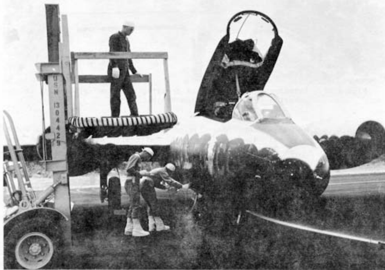
Figure 37. Crews prepare to decontaminate a B-57 sampler after crew and sample removal, Naval Air Station, Barbers Point, Operation DOMINIC.
