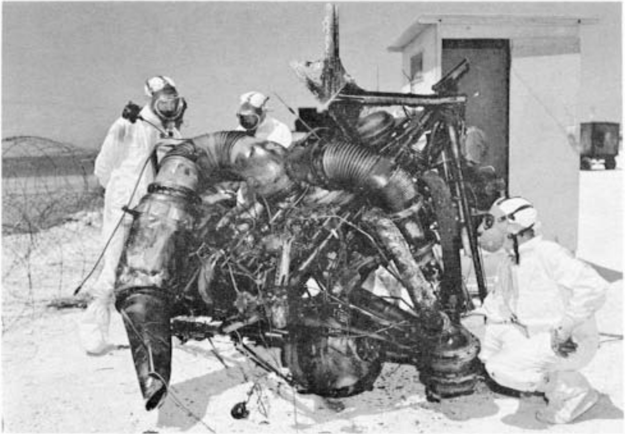
Figure 98. Inspection of Thor engine parts following BLUEGILL Prime fire on Johnston Island, Operation DOMINIC.
