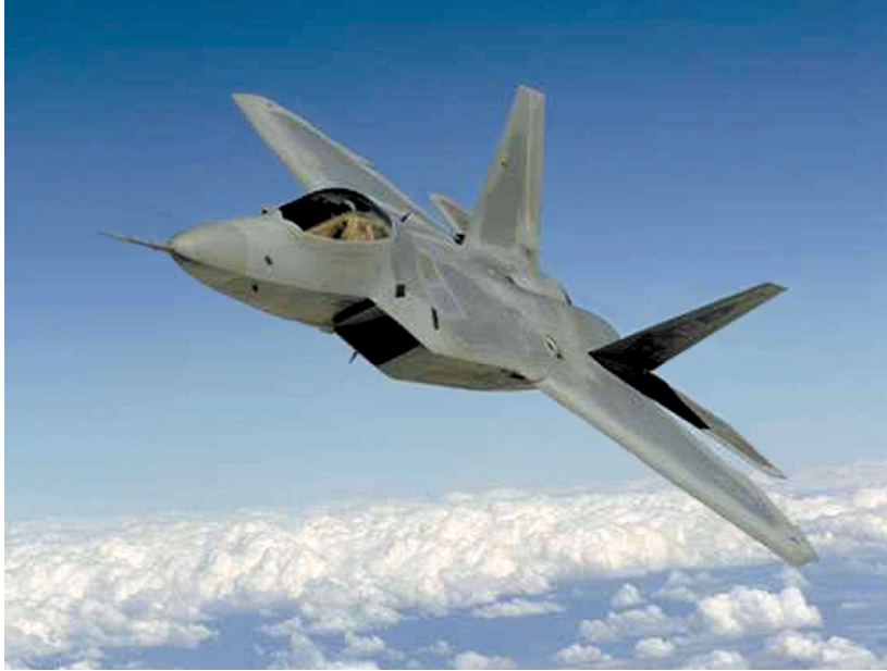
The F-22 “Raptor” stealth fighter, above, has been outfitted with special technologies, such as leading-edge cooling and special surface paints, for infrared signature reduction at high-speeds.
