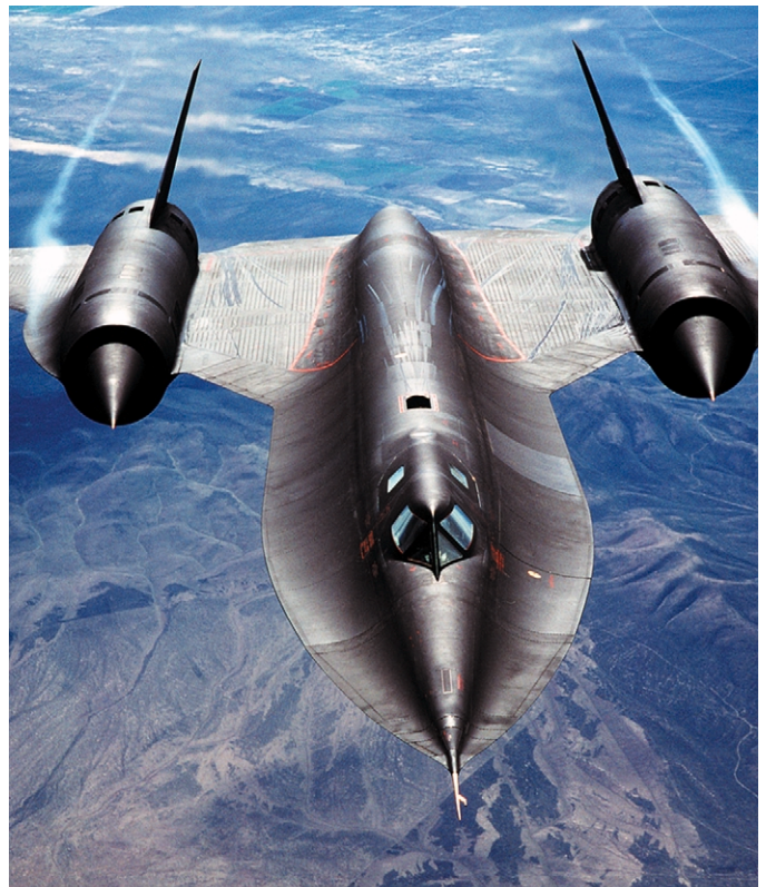
The Lockheed SR-71 Blackbird, above, was the first military aircraft designed from inception to minimize radar cross-section.
