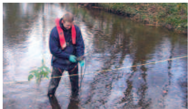
Hydrometric gauging in the Bollin catchment
