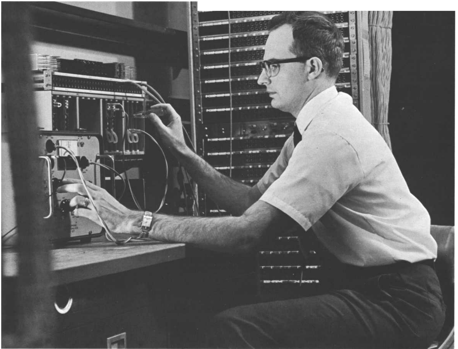
T. A. Sickman of Bell Laboratories tests and adjusts equalizers to be used in Picturephone loops. The equalizers are connected to a 6000-foot length of test cable to simulate a customer loop arrangement. In addition to providing gain compensation, equalizers are used to correct distortion of the video signal.
