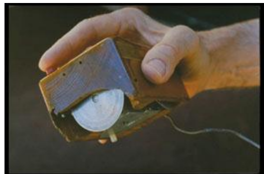
Figure 9 The first mouse was a wooden case of 2"x3"x4", about 5x7.5x10 cm, mouse was the name given to the device in the laboratory, due to its aspect. 6
