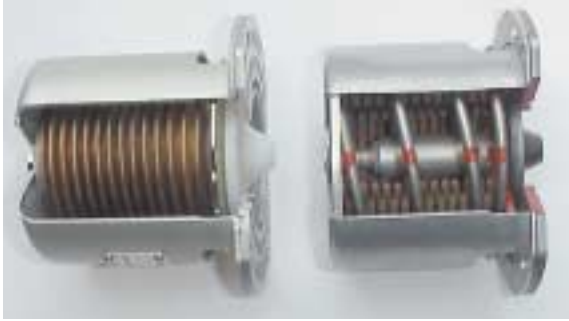
Two styles of PRVs. The valve on the right has an external non-damped spring which is a separate part surrounding the bellows. The valve on the left is designed for high-vibration environments. The spring is encased within the bellows assembly that is partially oil-filled to provide vibration damping.
