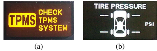
Figure 16: Dash panel snapshots indicating the TPMS system error (this error cannot be reset without the help of a dealership): (a) the vehicle’s general-information warning light; (b) tire pressure readings are no longer displayed as a result of system function errors.
