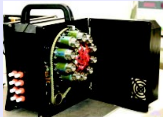
Instrument to detect extant life (SOLID, from Spain) at TRL 5.
