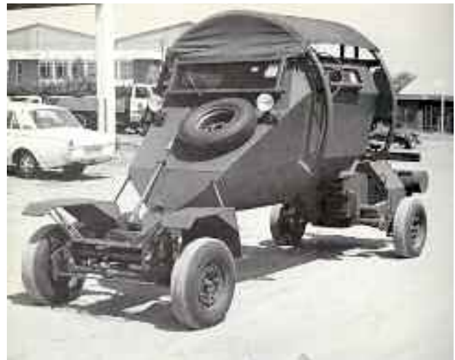
Figure 6. The Leopard. It incorporated the V-shaped hull with the single monocoque hull which provided protection to the drive-train as well as the passenger compartment. The increased axle length brought the wheels outside the passenger compartment and the easily sheared connection meant that the wheel assembly would be blown clear of the vehicle if it detonated a mine. (Source: Ernest Konschel. Available from: http://www.baragwanath.co.zalleopard/ )
