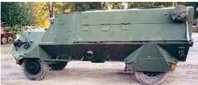
Figure 5. The Swedish SKPF M/42 Armoured Personnel Carrier developed during WW2 was the first vehicle to incorporate the V-shaped hull to aid deflection of the detonation products. This feature was later included in both Rhodesian mine vehicles and in modern coalition mine-protected vehicles.
