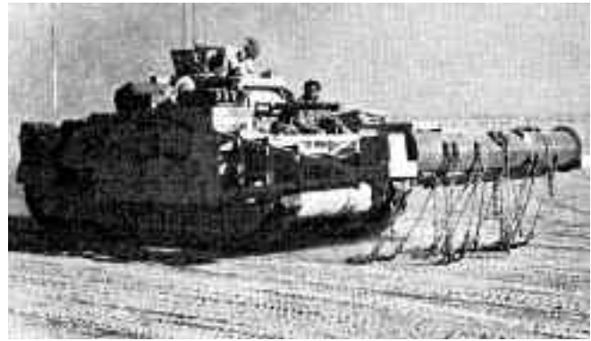
Figure 4. The Matilda-Scorpion Flail Tank. The Flails were designed to detonate the mines in order to create a clear passage through a mine field.
