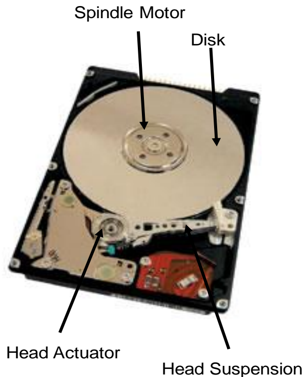
Figure 5. Illustration of hard drive components.
