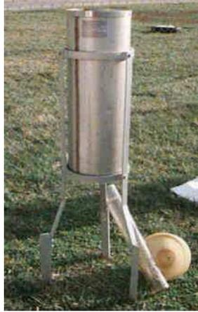
Figure 1.1: The National Weather Service Standard Rain Gauge, SRG (source: [http://www.srh.noaa.gov/tlh/cpm/srg\\_page.html](http://www.srh.noaa.gov/tlh/cpm/srg_page.html))
