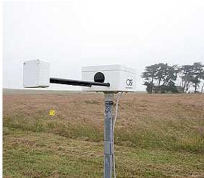
Optical rain gauge (source: The Atmospheric Radiation Measurement (ARM) Program)
