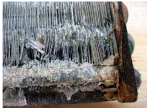
Figure 2 – RTPF Coil with 1 Year of Exposure
