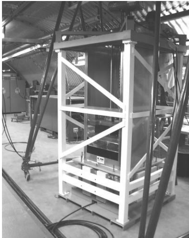
Figure 9. EMML Launcher structure, canister, propulsion coils, armature and weighted adaptor
