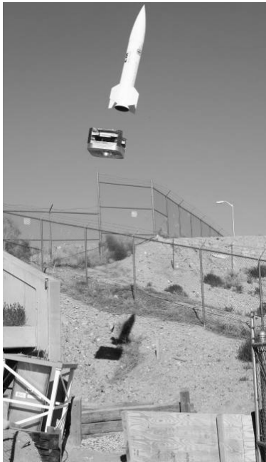
Figure 1. Demonstrator launcher; Launcher – bottom left; Weighted sled and missile form – top middle
