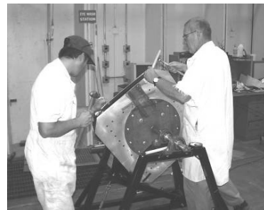
Figure 7. Winding coil on spool
