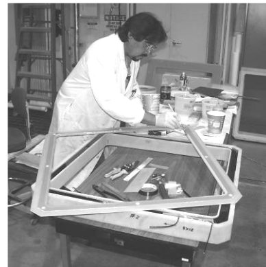
Figure 8. Applying adhesive to bond lid on outer coil
