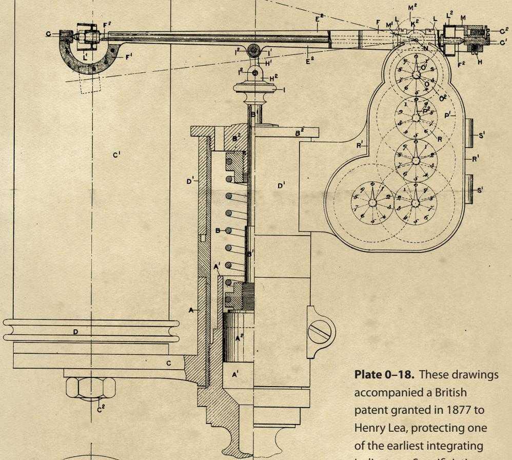
**Plate 0-18.** These drawings accompanied a British patent granted in 1877 to Henry Lea, protecting one of the earliest integrating indicators. Specifications of this type are among the most useful reference tools. *Courtesy of the UK Intellectual Property Office, London.*
