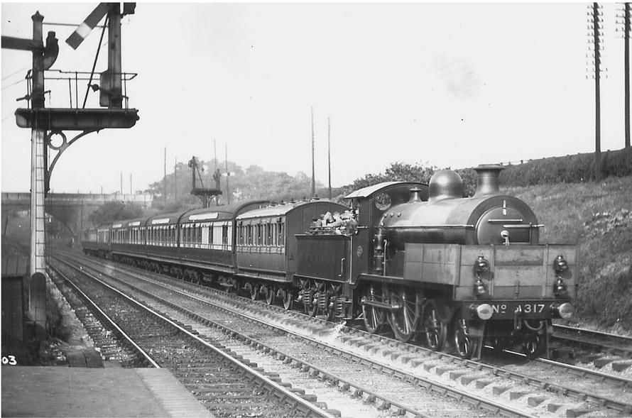
**Plate 0-17.** The introduction of the autographic indicator allowed the performance of steam engines to be assessed under many conditions. The wooden hoarding on the running plate of this London, Brighton & South Coast Railway locomotive, photographed in the early years of the twentieth century, protected engineers endeavouring to take diagrams at high speed!. *John Walter collection.*
