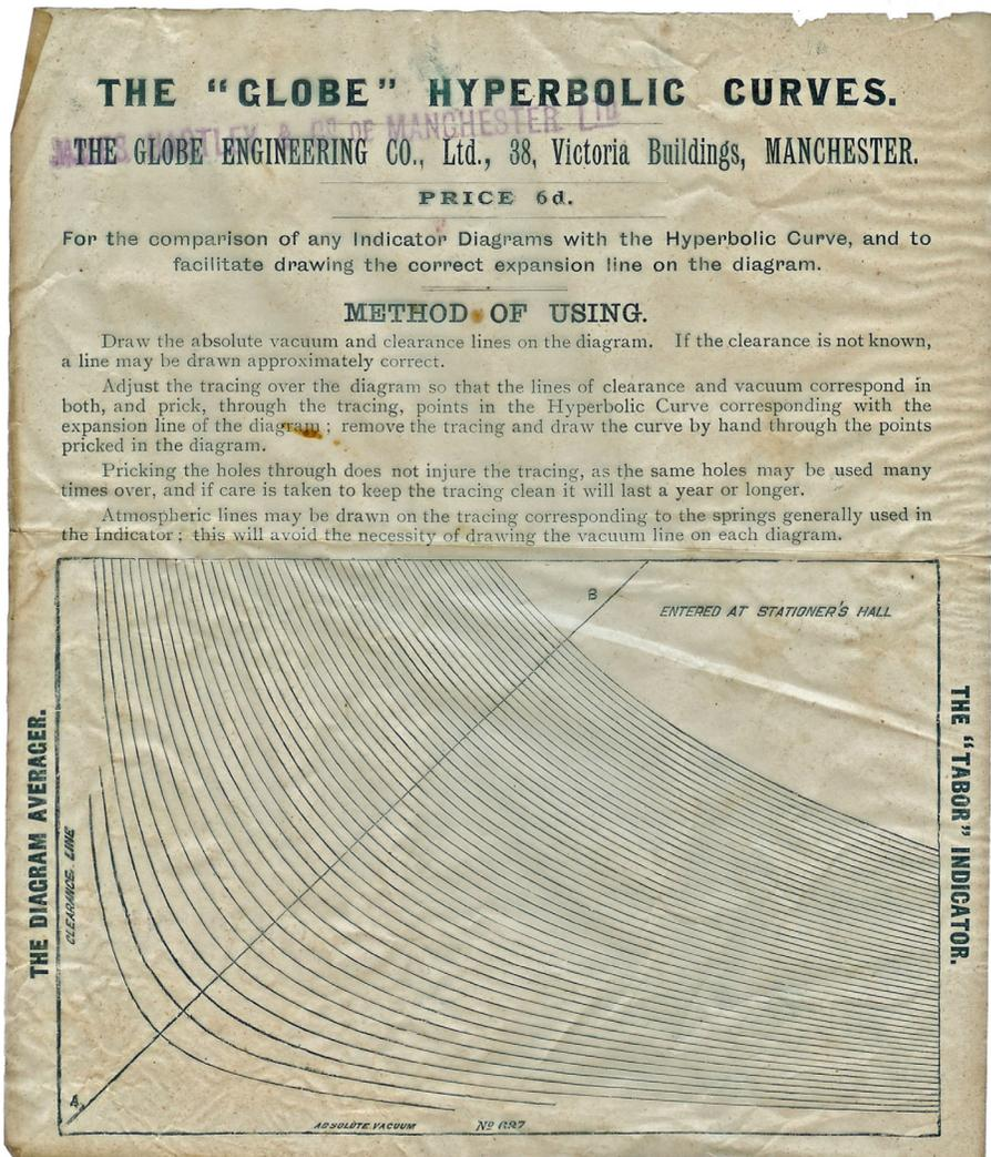
**Plate 0-15.** Printed on translucent paper, this was prepared partly as a promotional tool (Globe briefly distributed Tabor indicators in Britain) and partly to provide a method of comparing actual performance with thermodynamic theory. *John Walter collection.*
