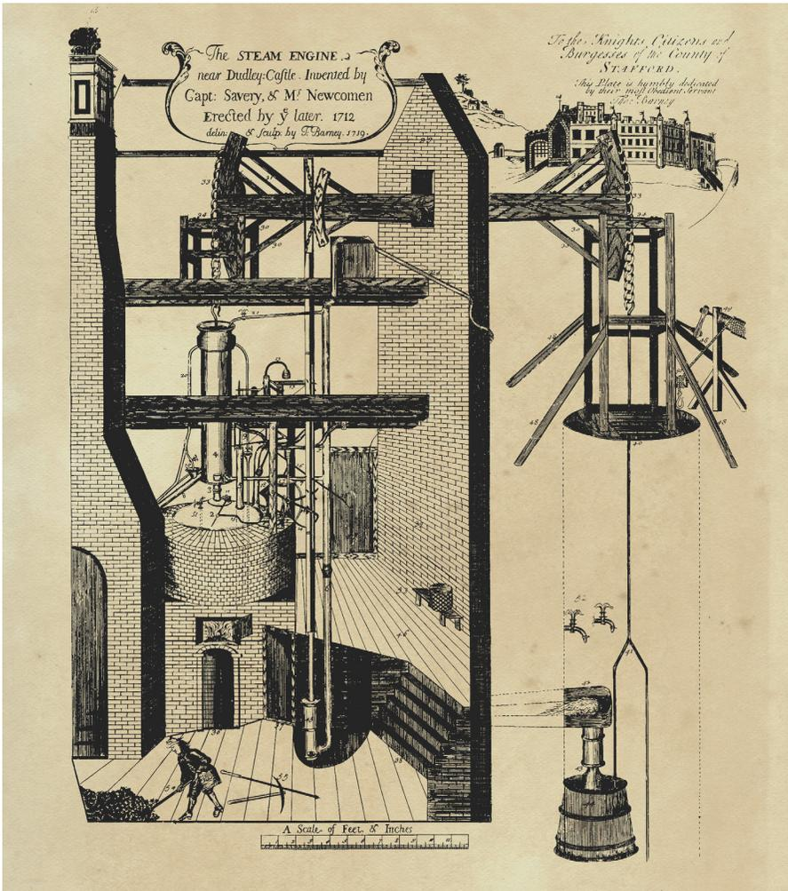
**Plate 0-1.** This reproduction of an engraving by Thomas Barney, originally dating from 1719, is the earliest known illustration of a Newcomen atmospheric engine—in this case, the so-called ‘Dudley Castle’ engine erected in 1712. *John Walter collection.*
