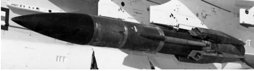
Figure 7. Advanced Low-Volume Ramjet flight test vehicle (ca. 1975).
