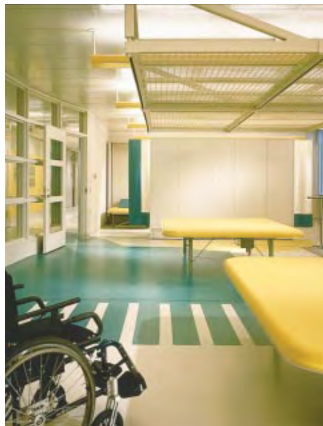
Therapy areas used indirect fluorescent pendants with perforated bottom channels to soften contrast.
