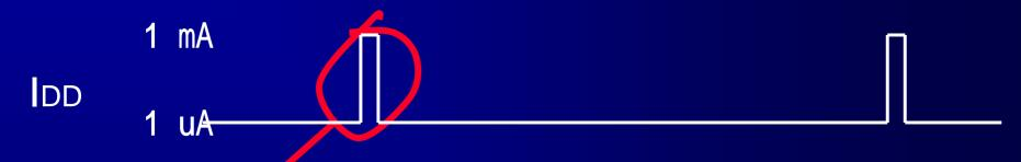
Device wakes up, test a condition and go back to sleep
