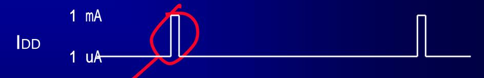
Device wakes up, test a condition and goes back to sleep For Battery Applications:
