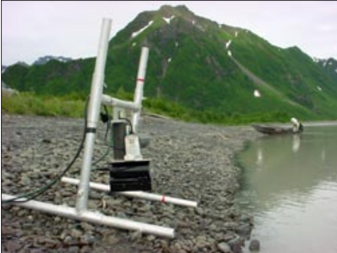
FIGURE 2. — A dual-frequency identification sonar (DIDSON) system.
