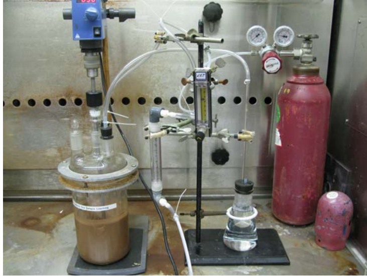
Figure 11: Stirred Tank Leaching with SO 2 /N 2
