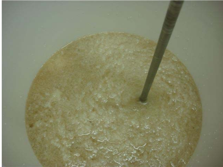
Figure 21: Initiation of \text{MnCO}_3 Precipitation with the Addition of \text{Na}_2\text{CO}_3
