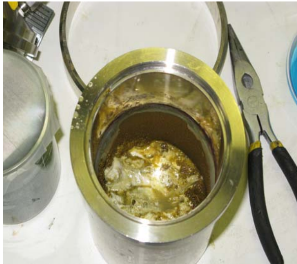
Figure 33: Precipitate obtained during the autoclave testing
