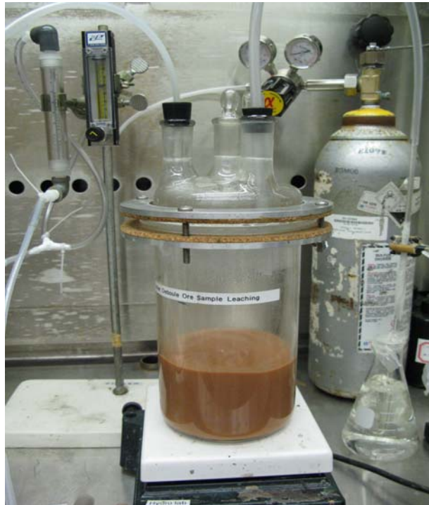
Figure 10: Experimental Set-up for Manganese Extraction with SO 2 /N 2 Mixture
