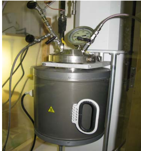
Figure 32: Autoclave set up for high temperature and pressure oxidation
