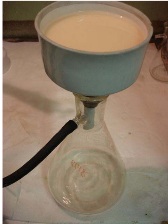
Figure 23: Filtration of the MnCO_3 Precipitate
