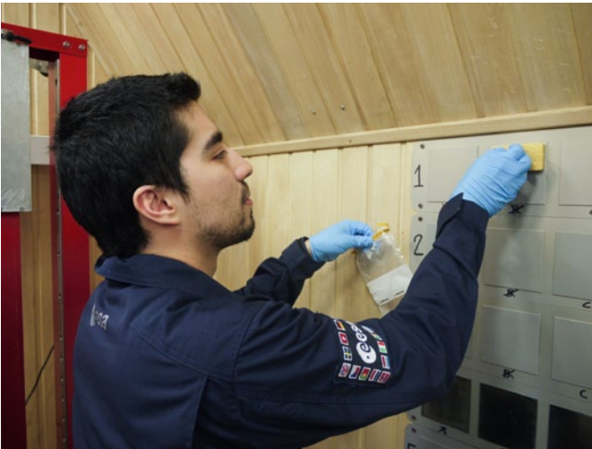
Diego Urbina is collecting microflora samples from the panels, used in the orbital modules of the space station
