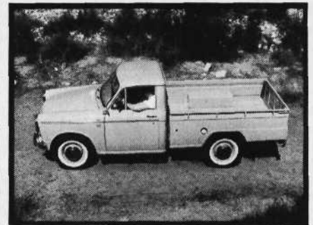
4-speed transmission and powerful 60 H.P. engine gives amazing power. Big 6' x 4'8" bed carries up to 1 ton.
