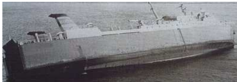
Free surfaces on board always increase the risk of capsize.
