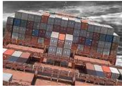
Rolling is the movement of a ship around its longitudinal axis, the rolling angle in this case being 10°.
