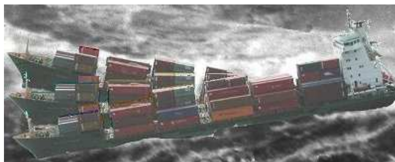
Pitching is the movement of a ship around its transverse axis
