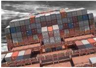
Rolling is the movement of a ship around its longitudinal axis, the rolling angle in this case being 10°.
