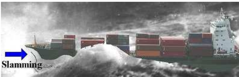
Slamming describes the hydrodynamic impacts undergone by a ship
