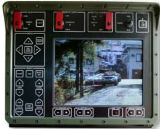
Fire Control Unit (FCU)
