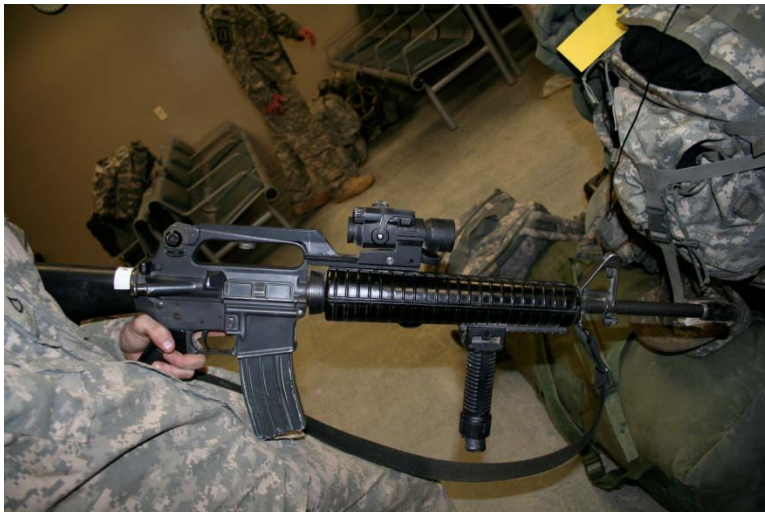
M16A2 with M68 CCO and bipod mounted...no M1913 Rails.
