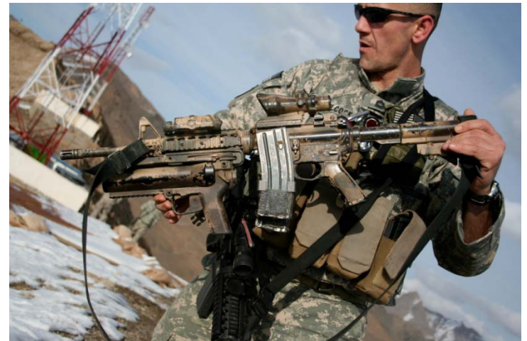
M320GL mated to M4 Carbine...weapon painted, no sights for M320GL
