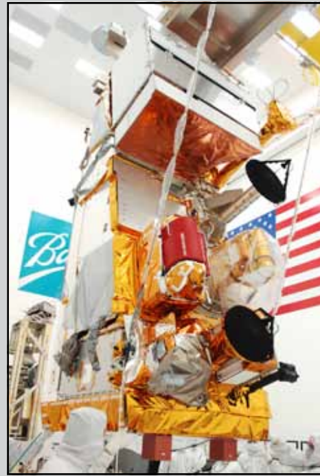
The NPP spacecraft is a modified BCP 2000 bus, shown here being transported to its workstand.
