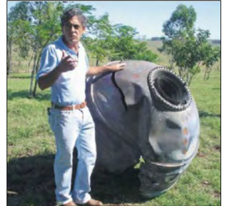
Figure 1. STAR-48B motor casing which landed in Uruguay during the evening of 2 March 2011 (local time).
