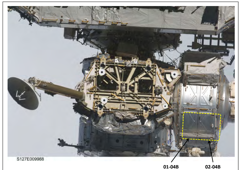
Figure 1. The ISS airlock module on right side, zenith view. Yellow dotted lines indicate the two exterior shield panels that were removed and returned to Earth for inspection. Panel 01-04B is the inboard panel and 02-04B is the outboard panel. The ISS velocity direction in this view is toward the top of the page.
