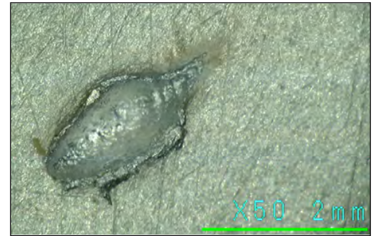
Figure 5. Non-circular crater found on the inboard panel (2.4 mm long x 0.9 mm wide).
