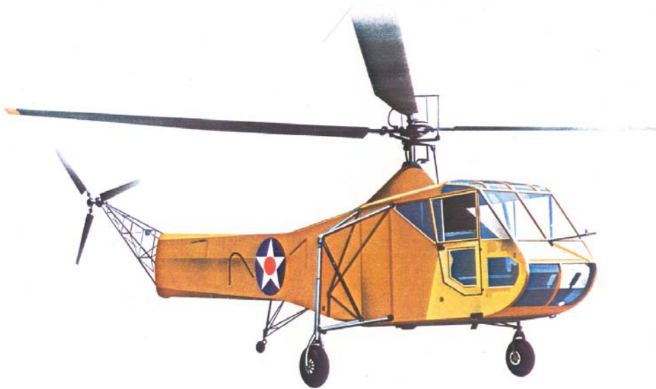
Sikorsky R-4, First Flight Jan. 1942 (Collective + Cyclic + VTOL )
