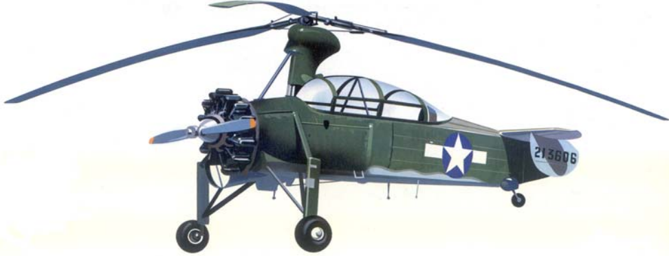
Kellett YO-60, First Flight Feb. 1942 (Collective + Cyclic + Jump Takeoff )
