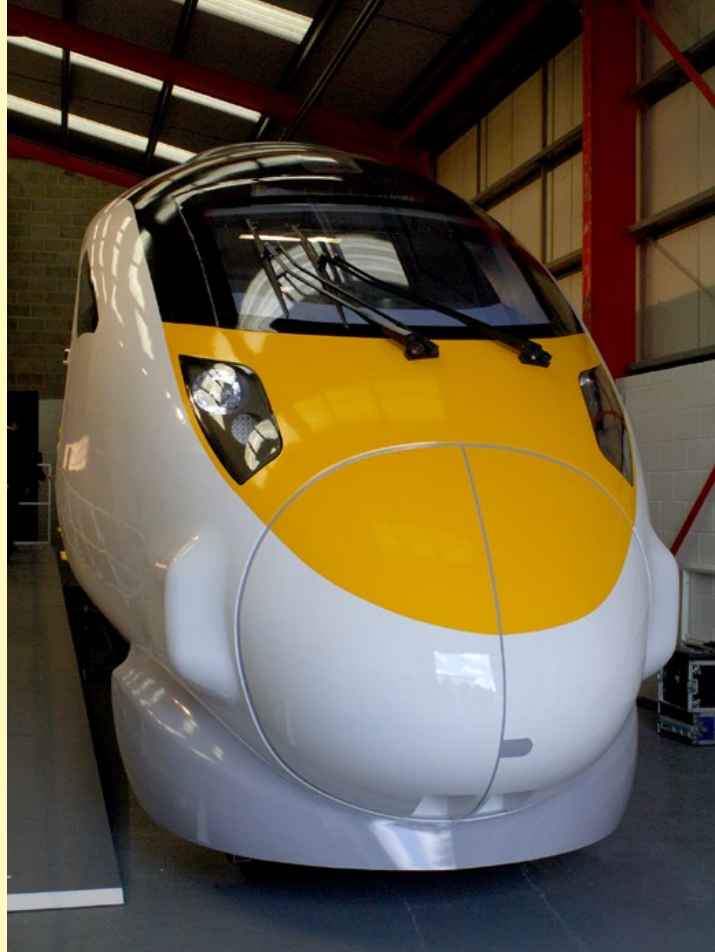
ABOVE: The very 'Bullet' style front end of the Class 395, incorporating a single cab window, with bi-parting front doors covering a Dellner coupling unit.
