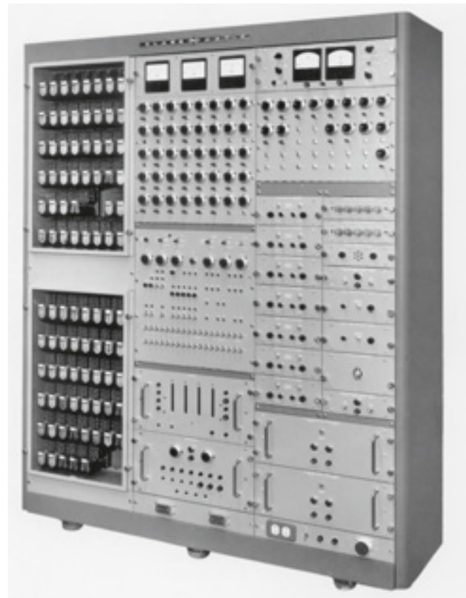
A GRS CLASSMATIC™ Analog Computer used in 1950's and early 1960's Yard Automation Projects.
