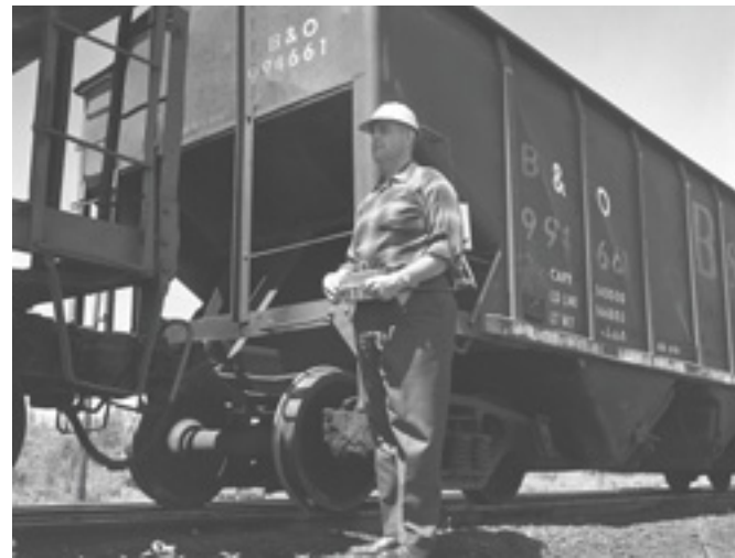
GRS radio remote control enables the operator to control his train from the ground.
