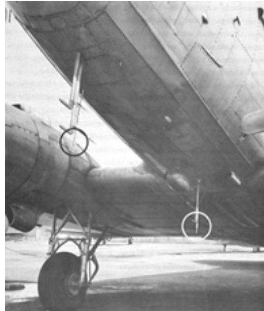
Air Traffic Control Master Control Station in Rochester (below), typical ATC Block Station in Albion NY (right), ATC aircraft antenna installations (above) in 1948.
