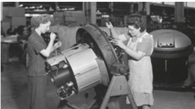
Remote control turrets for B29 bombers were made by GRS during World War II.
