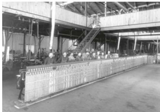
400 lever interlocking machine for Grand Central terminal on GRS factory floor in 1912.
