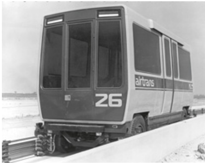
One of the AIRTRANS vehicles at the Dallas/Ft.Worth Airport which transports passengers between terminals in 1973.
