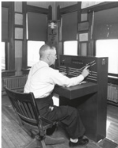
The first NX machine in the US was placed in service later in 1937 on the New York Central at Girard Junction, Ohio.
