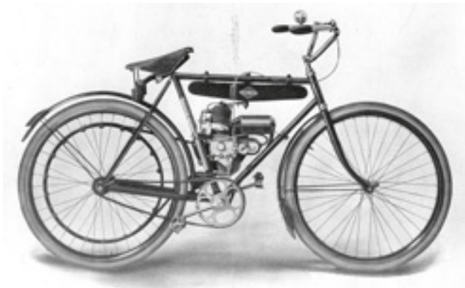
The Cyclemotor as applied to an ordinary diamond-frame bicycle.
