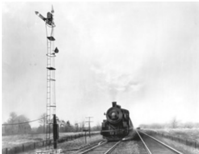
GRS intermittent inductive train control was tested on the Buffalo, Rochester & Pittsburgh Railway in 1919.
