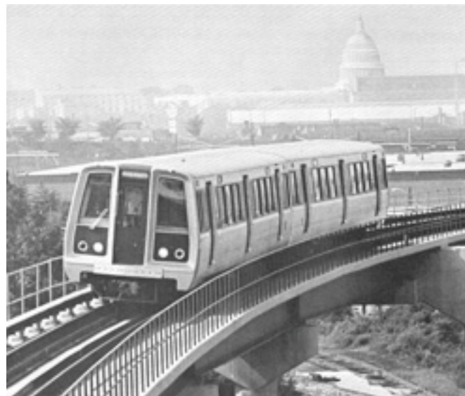
In 1976, the first section of the Washington Metro was equipped with a GRS fully automatic train control system which permits trains to operate up to 70 mph with 90-second headways.
