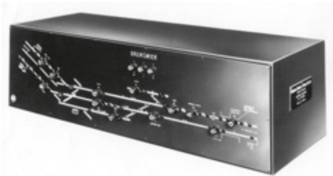
Heralding the approach of the pushbutton age, this GRS NX interlocking machine (the world's first) was placed in service in 1937 at Brunswick, England.
