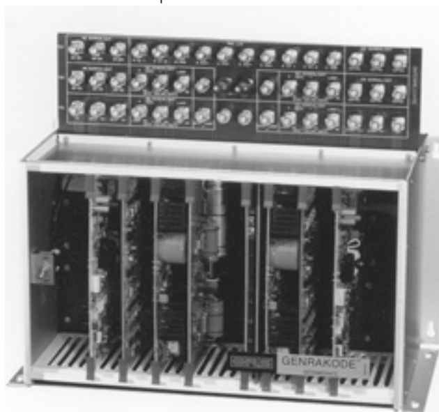
GENRAKODE is one of the latest vital processor based wireless block signal and track circuit products from GRS.
