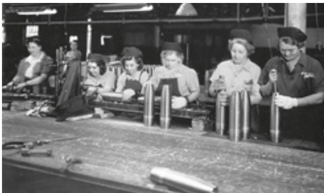
Country's first completely power-conveyorized system speeds assembly of 105-mm shells in World War II.
