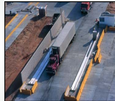
Relocatable Vehicle and Cargo Inspection Systems (RVACIS)
