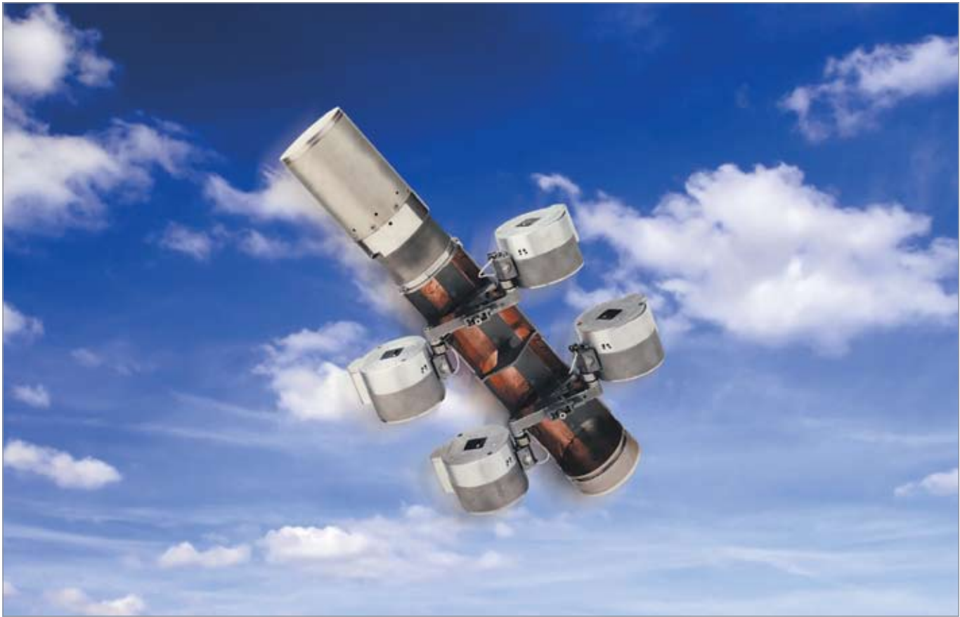
The BLU-108 parachutes to near the ground and releases four Skeet warheads [Textron Defense Systems]
