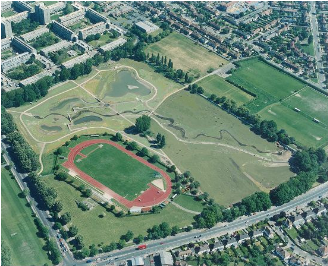
Figure 6.4 – Flood Storage Area – Upstream Storage
