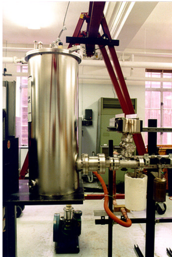
Fig. 8. Portable antiproton trap during testing.
