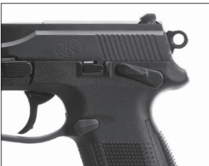
Hammer decocked for double-action firing
