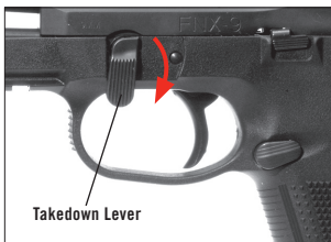
Rotate the takedown lever downward.
