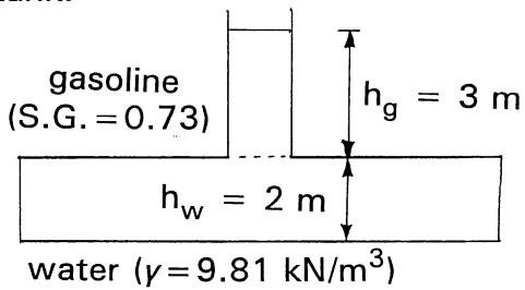
pressure at bottom of tank
