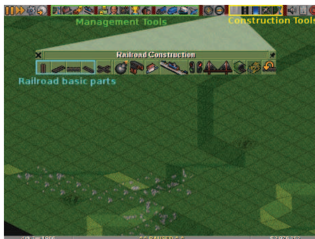
Figure 2: An OpenTTD screenshot: there two rectangles highlighting some tools available on game menu. The yellow tools predominantly have construction functions. By contrast, the green tools are essentially used for management tasks. It also shows the railway construction tools (the window positioned near the middle). The basic parts provided by the game for railroad track construction have been highlighted using the cyan color.
