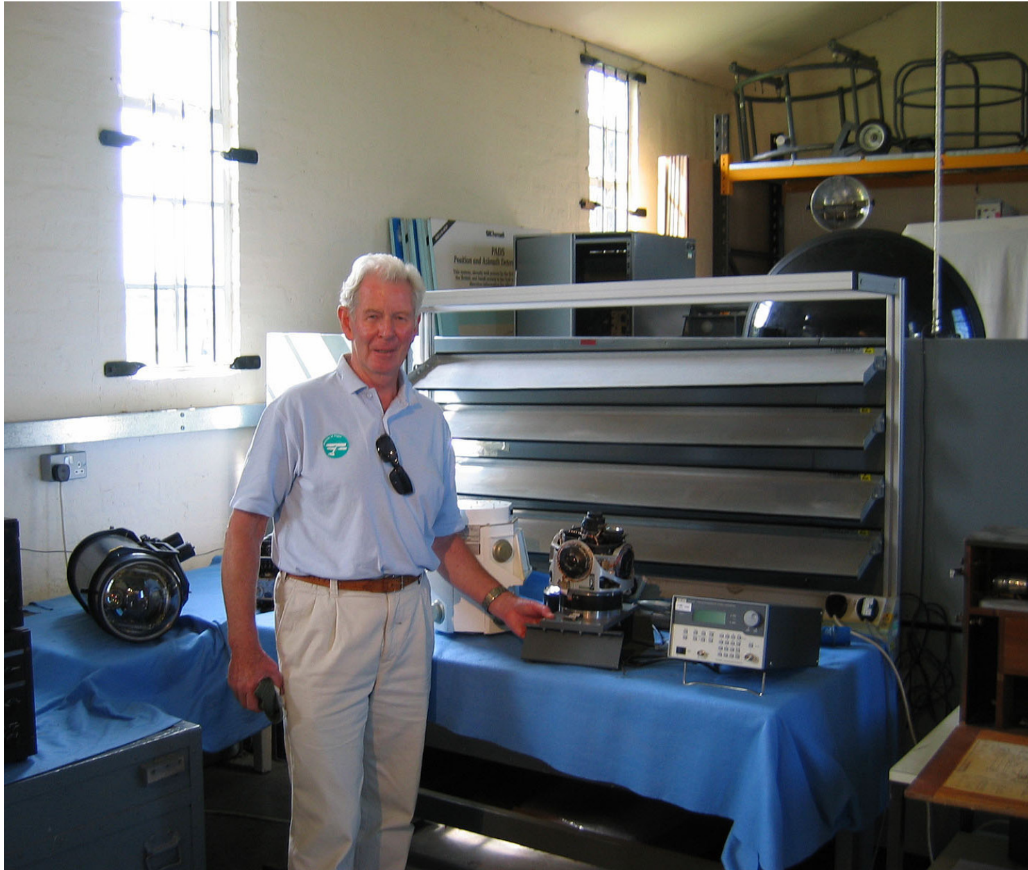
Seen a few years after the TSR.2's cancellation, our contributor Bill Blain is pictured with the Ferranti Laser Ranger and Marked Target Seeker (LRMTS) head, which went on to equip Jaguar, Harrier, and, later, Tornado ADV aircraft of the RAF.
