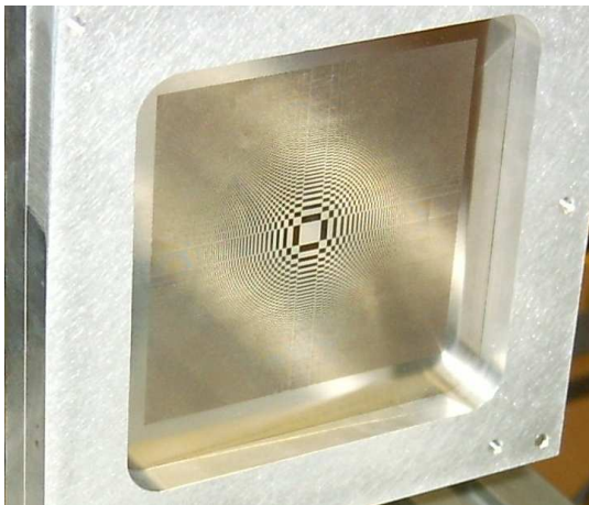
Fig I-3: 80 mm square Fresnel primary array carved into a thin 80 \mu\text{m} stainless steel foil, used for optical tests. (58 Fresnel zones, 26 680 subapertures).
