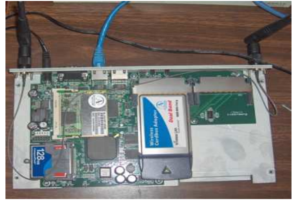
Fig. 9. Picture of a testbed node. Each testbed node is equipped with two wireless interfaces.
