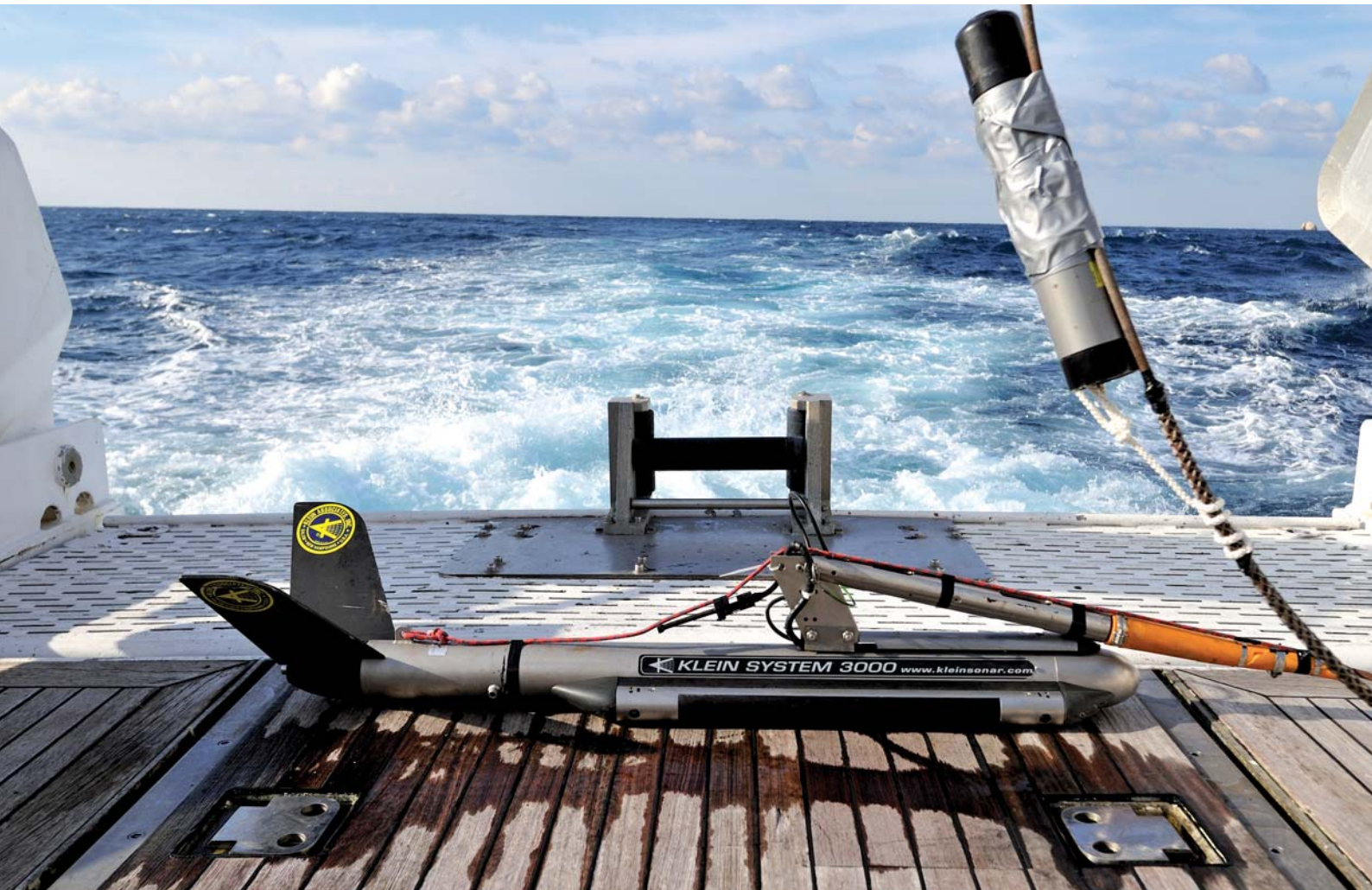
Side-scan sonar used to map seabed
