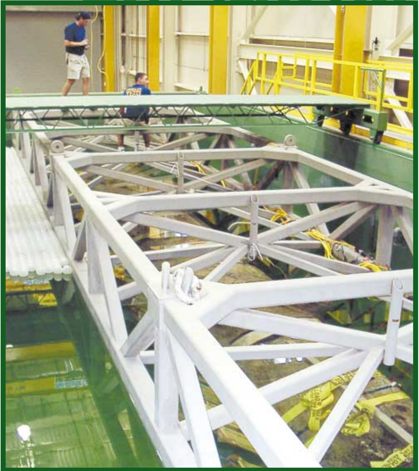
A truss of HSS helped raise the Civil War submarine Hunley from the ocean floor.
