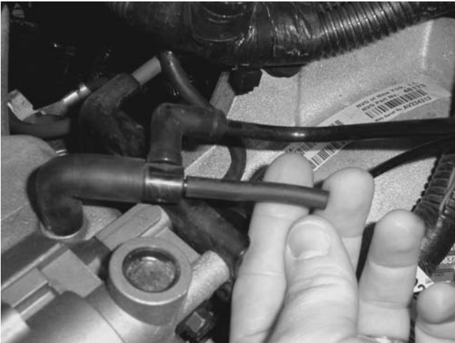
Fig. 3 Vacuum Tee Installation
