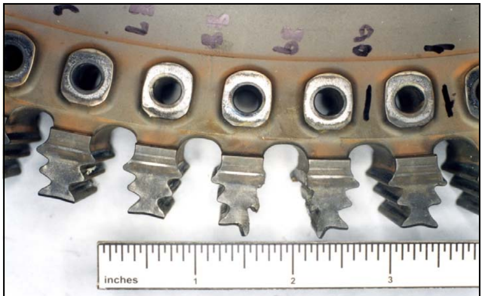
Figure 2. Long-term aging and metallurgical deterioration were the underlying causes of a turbine wheel-post failure that allowed a blade to release into the flow path.
