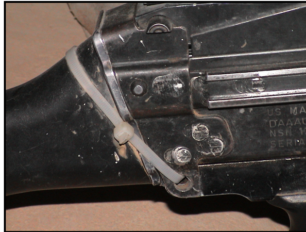
Figure { SEQ Figure \* ARABIC }. M249 SAW with field expedient repair.
